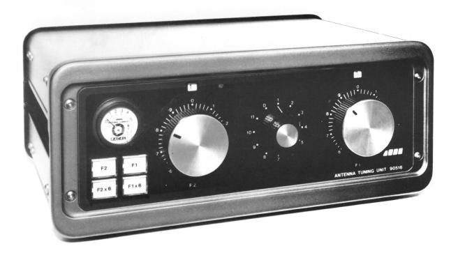
The Antenna Tuning Unit type 90516 is a lightweight, compact, dual frequency tuning unit designed to match the PA into antennae from 3 m to 30 m over the frequency range 1600 kHz to 3400 kHz.
