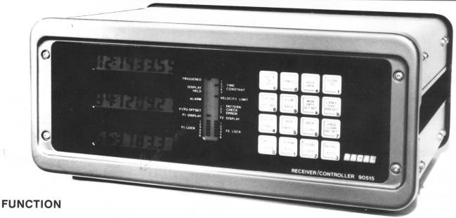
The Hyper-Fix Receiver/Controller has the dual function of shipborne (or monitor) receiver and shore station control unit. Selection of the required configuration is made from the keyboard when the unit is first switched on and initialised. At this stage, the unit is designated as CONTROLLER or RECEIVER and remains in this mode until re-initialised.
