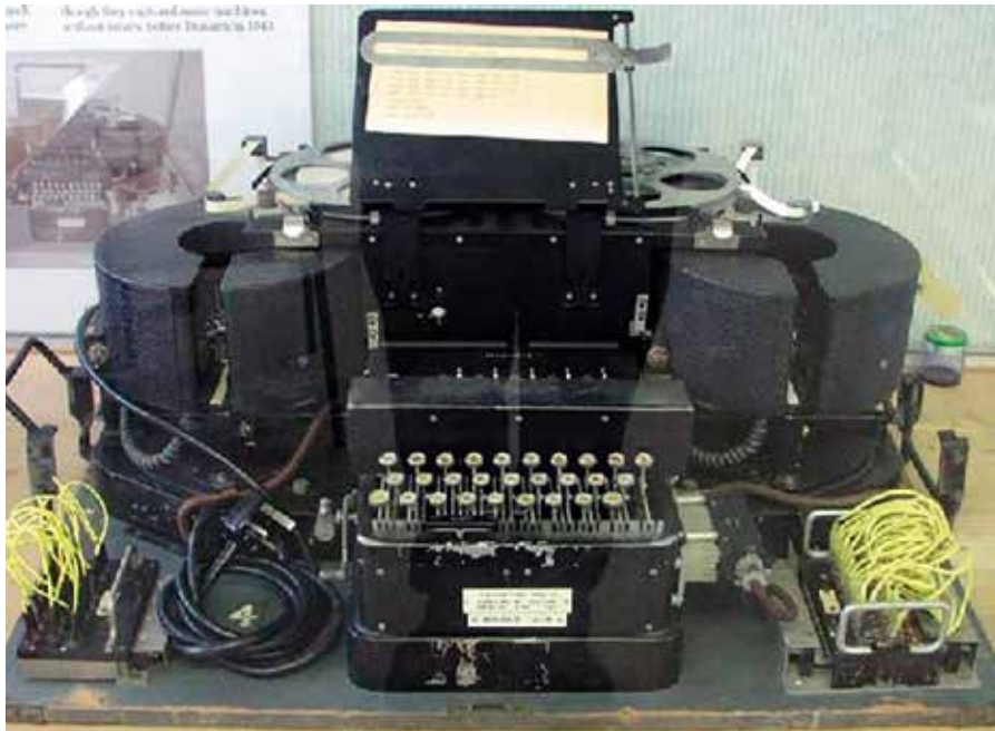
Fig. 8. Typex Mk 22 cipher machine. It employed five rotors and one reflector plus plugboards. A good operator could key the machine at 40 wpm. (Bletchley Park photo via Wikipedia)
