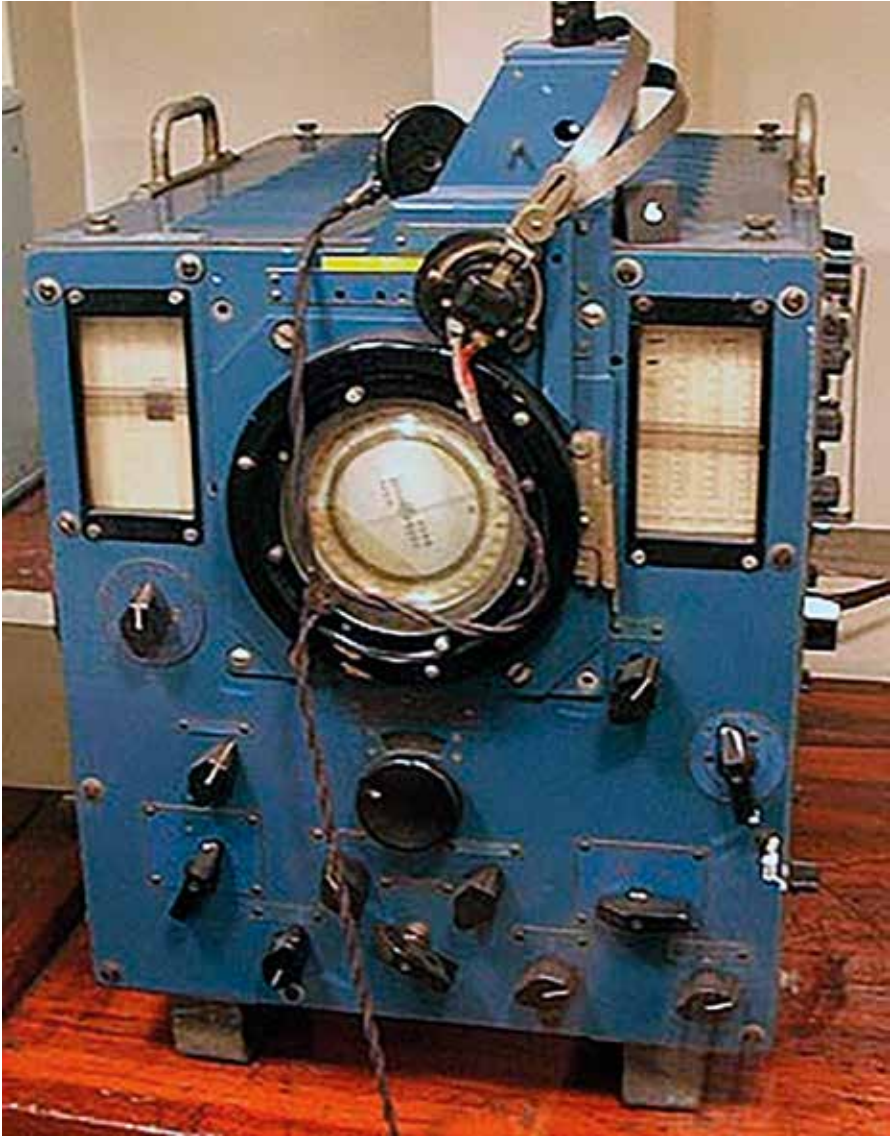
Fig. 3. The FH-4 HF/DF could tune the range of 1 to 25 MHz. (Photo by Øyvind Garvik)
