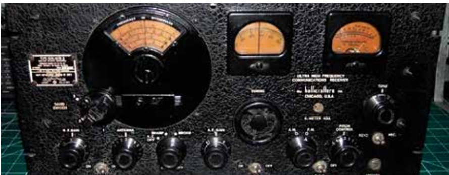
Fig. 6. German VHF aeronautical frequencies were monitored using receivers like this Hallicrafters S-27 ultra high frequency communications receiver. (Photo courtesy UK Vintage Radio web page)
