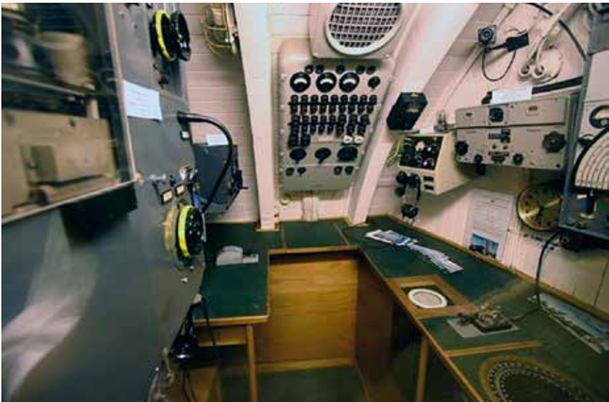
Fig. 5. This is the very cramped radio room of the German submarine U-995. What is missing is the famous Enigma machine. (Photo courtesy Uboataces.com)
