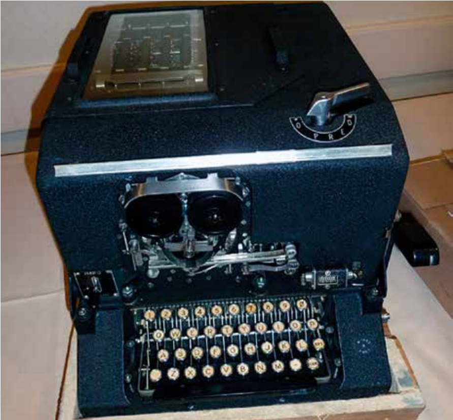
Fig. 10. The American ECM Mk II cipher machine was also known as SIGABA. (Photo by Ralph Simpson)
