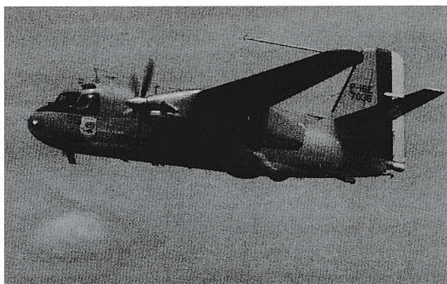
Grumman S-2E (P-16E) 7036 of the Força Aérea Brasileira following conversion by the IMP Group to turbine engine configuration. The FAB subsequently cancelled the programme to convert its fleet to P-16Hs. (IMP Group)
