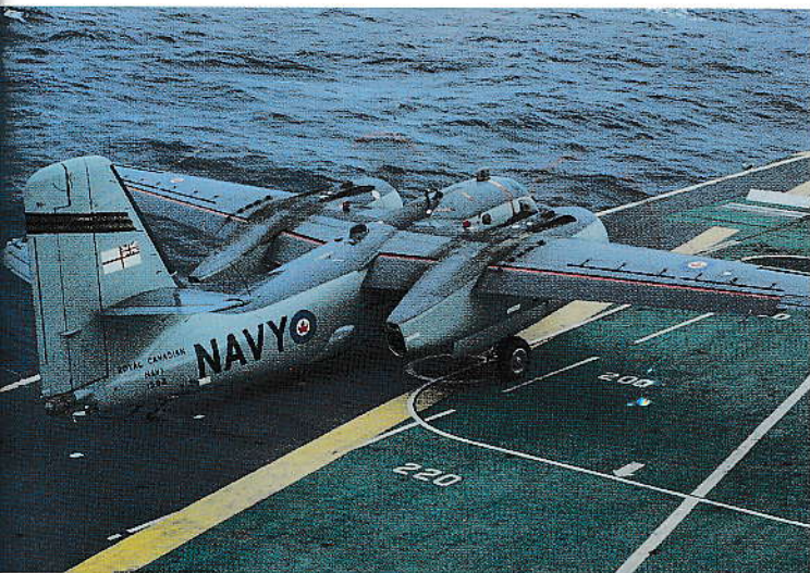
Heavily-loaded CS2F-2 1592 taxis tail-low towards the Bonaventure's catapult. The hold-back cable, visible behind the tail bumper, was designed to fracture with the aircraft at full power and with sufficient tension from the catapult. This aircraft was lost on February 16, 1969, when the launch bridle failed during the launch, sending the luckless Tracker over the bow before reaching flying speed. The crew, including the co-pilot who passed through the ship's propellers, was rescued by the Sikorsky HO4S plane-guard. (Seth Grossmith)
