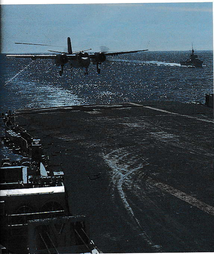
Tracker 1532 of VX 10 makes a textbook approach while the plane-guard destroyer stands by. The source lights for the primary Mirror Landing System are visible to the right. (Seth Grossmith)
