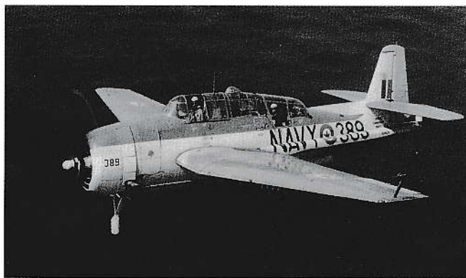
The Royal Canadian Navy's AS.3M Avenger represented the ultimate development of the single-engined Grumman design in the anti-submarine role. The MAD boom sleeve and front and aft ECM cans are clearly visible in this view of 53908, call-sign '389'. (DND via Stuart Soward)
