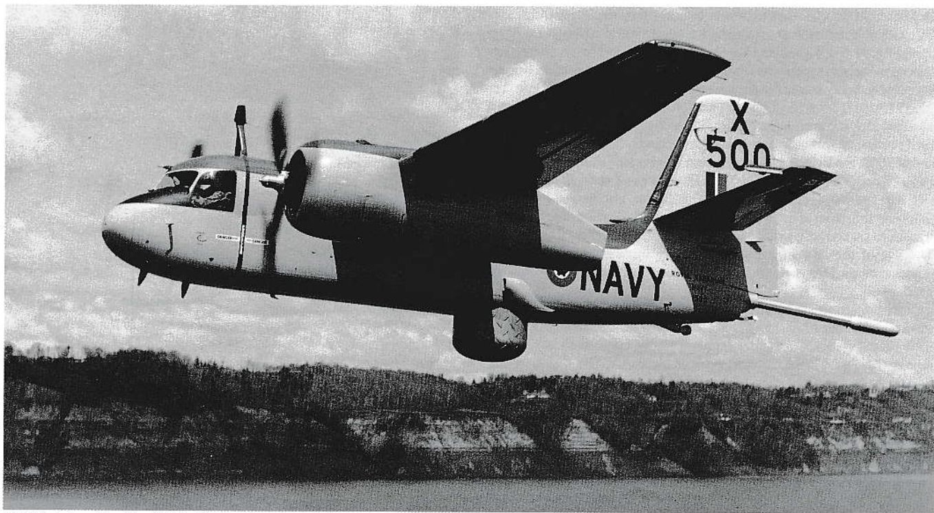
X-500 pictured in May 1955 after repainting in RCN colours with the addition of serial 1500. This early production Grumman S2F-1 Tracker was fitted with the dorsal mast for the US Navy-style bi-pole AN/APA-69 ECM direction finding antenna (though the actual ECM equipment was not installed) and is shown with its MAD boom and ventral radar antenna radome extended. As first designed, the radome caused two problems when lowered for ASW operations; excessive drag and aircraft instability around the vertical axis. To address the drag, Grumman added a scoop with a narrow horizontal outlet nozzle to each side of the aircraft, just above the radome; the net effect was to smooth the airflow to the rear of the radome and restore some of the lost performance. The directional 'hunting' and an associated trimming problem were resolved by adding the vortex generators visible on the side of the radome. (de Havilland Inc.)
