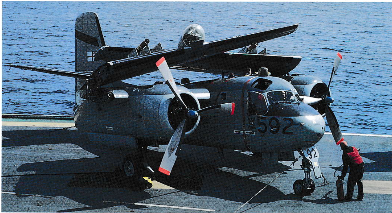
CS2F-2 1592 just prior to start-up aboard HMCS Bonaventure. Note the hold-down chains and the plucky chock-man laying beside the starboard mainwheel. The aircraft carries air-droppable life raft canisters on each of its centre underwing pylons. (Seth Grossmith)
