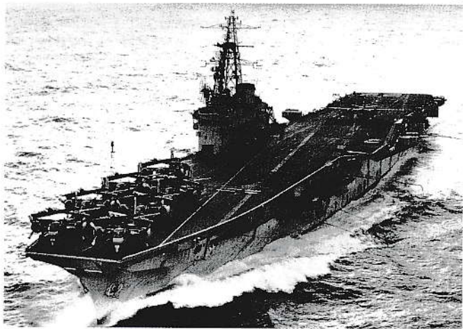
HMCS Bonaventure recovers one of its early complement of anti-submarine CS2F-1 Trackers. The new angled-deck allowed landings to take place while inactive aircraft remained stored on the forward deck. The two sets of catapult chocks are visible to the right of the parked aircraft. (DND)
