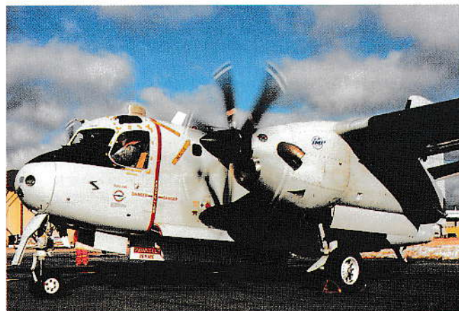
The IMP Group converted a single CP-121 Tracker to turboprop configuration based on the P&WC PT6A-67AF. The flared forward nacelle for the R-1820 'round' engine remained unmodified so the aircraft could be converted back to piston-engined configuration, resulting in the generous cowling. The Tracker's two-door port-side torpedo bay is shown to advantage. (IMP Group)
