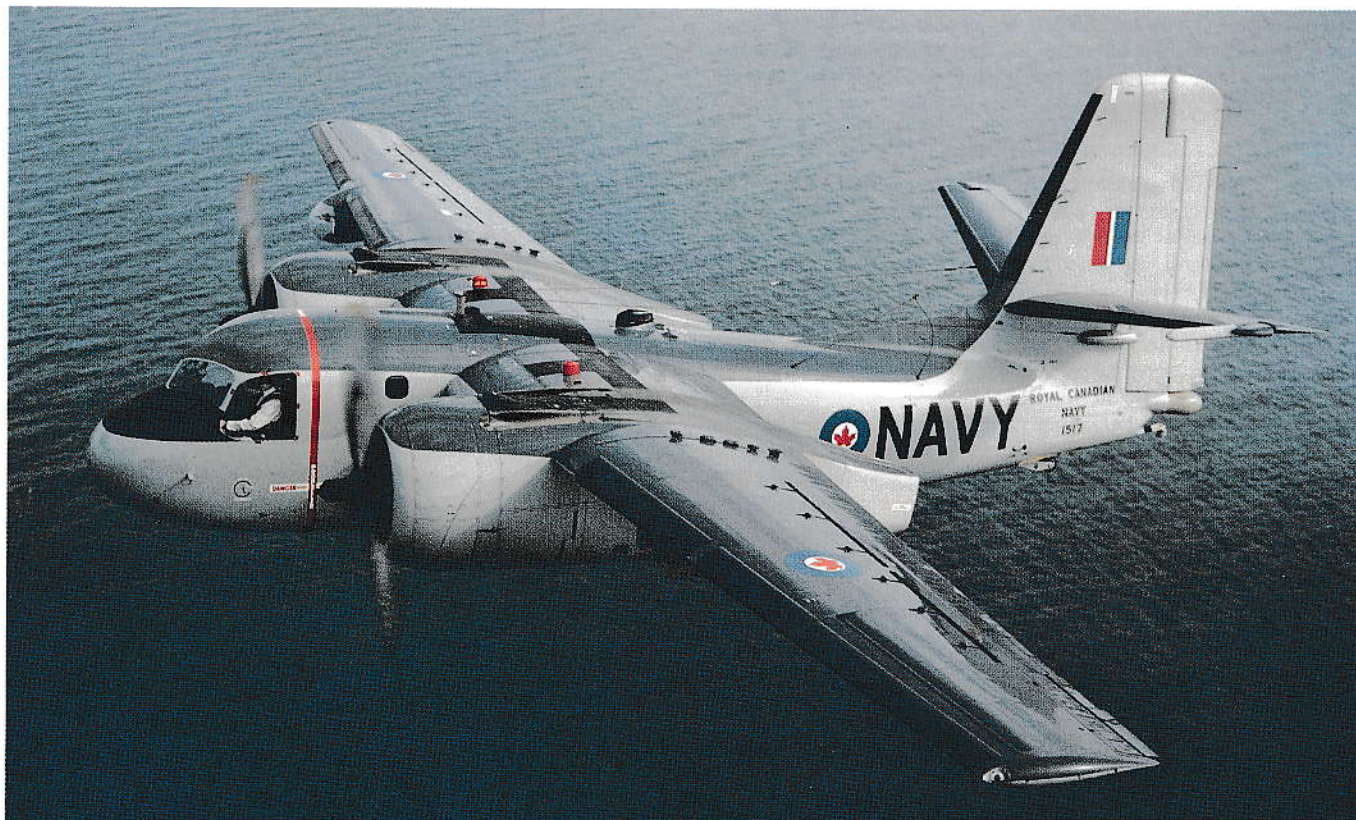
De Havilland Aircraft of Canada CS2F-1 Tracker 1517 prior to delivery in May 1957. Note the short span ailerons, the two slots in the upper surface of each wing for the roll control spoilers, the proportionately large vertical tail with its two-section control surface and the absence of transparencies in the pilots' overhead escape hatches. This Tracker had a relatively short naval career being written off in January 1960. (de Havilland Inc)
